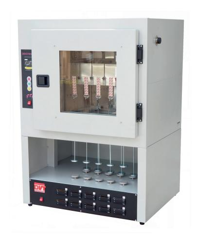
USED TO TEST STATIC SLIDING ADHESION IN ADHESIVE BANDS
